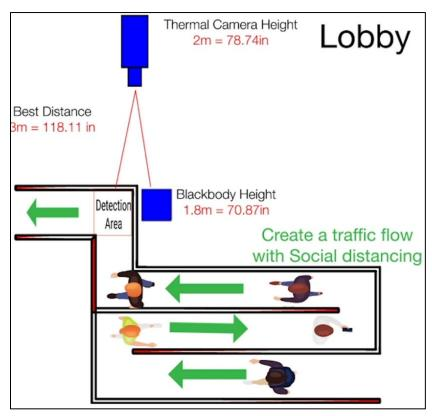
Figure 2: Illustration showing optimal placement of components
