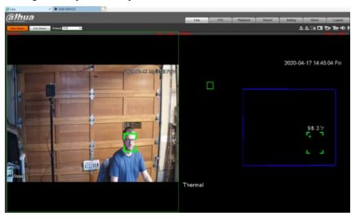
Figure 3 Left side represents the visual lens of the hybrid thermal camera with the temperature reading and the right side represents the thermal lens with a privacy protection mask.
